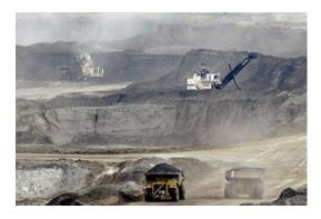
Oil sands are deposits of bitumen, a thick, tarry form of petroleum, buried deep beneath forests in Alberta. The bitumen needs to be extracted from the ground -- usually through strip mining or open-pit techniques -- and then processed to remove impurities before it can be used by refineries to produce gasoline and other fuels.
